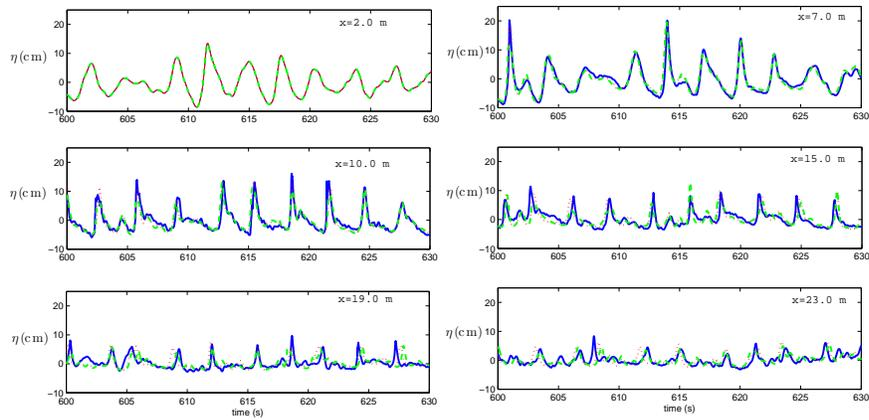
Figure 4. Time windows for measured and computed free surface at different spatial locations. (—) measured, (---) computed with CIEN model, and (· · ·) computed with KENN model.
