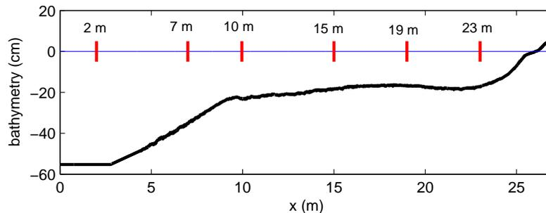
Figure 3. Bottom profile and wave gauge locations for the random wave experiment.
