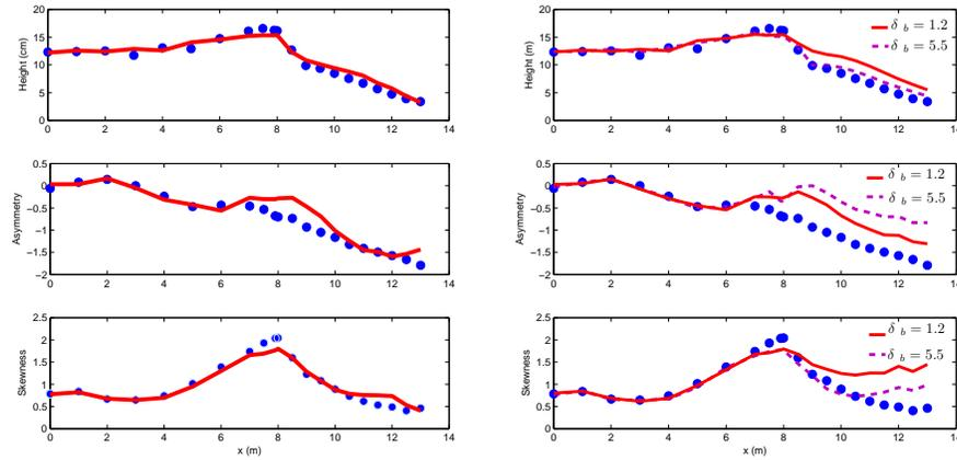
Figure 2. Comparison between measured ( $\bullet$ ) and computed ( $-$ ,  $--$ ) wave properties for Ting and Kirby (1994) experiment. Left panel: CIEN breaking model. Right panel: KENN breaking model.
