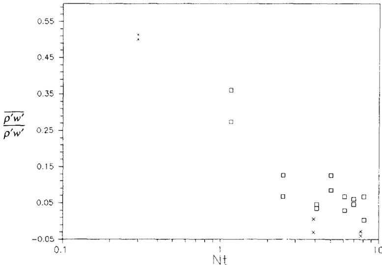
Fig. 6.  $w'$  and  $\rho'$  correlation, measured on the  $x$ -axis, as a function of  $Nt$ ; □,  $F = 10/\pi$ ; ×,  $F = 40/\pi$ ;  $Re(1) = 1218$ ,  $R = 2.5$  cm and  $N = 1.13$  rad  $s^{-1}$ .
