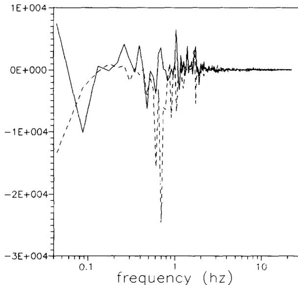
Fig. 9. Co-spectrum (solid line) and quadrature-spectrum (dashed line) between  $\rho'$  measured at  $z = 2R$  and  $z = 5R$ .  $x = 50R$ ,  $F = 6$  ( $\text{Re}(1) = 5474$ ,  $R = 5 \text{ cm}$ ).
