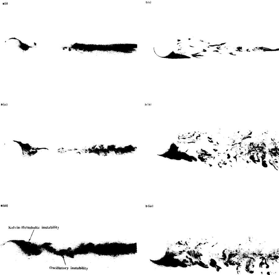
Fig. 1. Fluorescence induced by laser visualizations in (a) the vertical central plane, and (b) the horizontal central plane, for  $\text{Re}(1) = 1820$ . (i)  $F = 1$ ; (ii)  $F = 1.5$ ; (iii)  $F = 2$ .
