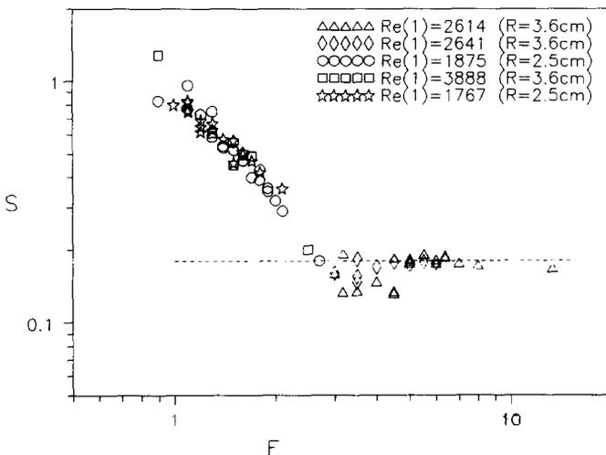
Fig. 2. Strouhal number of low-frequency instabilities of the wake as a function of the Froude number, determined from spectral analysis of velocity and conductivity probe signals. The probe is located at  $z = 0$  and  $x = 3R$ .
