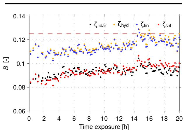
FIG. 3. Wave shape parameter  $B$  computed using the different reconstructed surface elevation signals and direct measurements from the lidar at PT2. The red dashed line corresponds to the  $1/8$  value.
