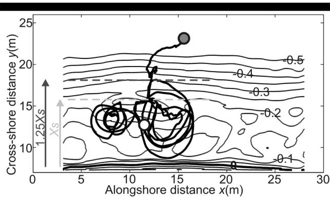
Figure 3. Example of a drifter pathline (thick solid black line) during video run d with the local bottom morphology contoured in the background (solid black lines) and with the white (grey) circle corresponding to the startup (end) of the pathline. The offshore extent of the semi-enclosed surf zone compartment is the dark grey dashed line with  $X_s$  the surf zone width.
