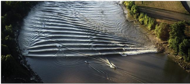
**Fig. 1.** Illustration of a tidal bore propagating in the Garonne River. Aerial photograph taken at Podensac on September 10, 2010. Tidal wave amplitude at the estuary mouth  $A_0 = 2.5$  m and freshwater discharge  $q_0 = 128$  m<sup>3</sup>/s.
