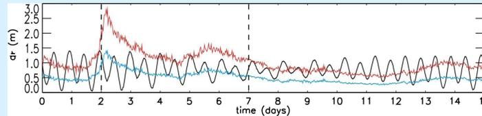
Fig. 3. Tide and wave conditions. Black line: mean water depth at the reef top  $d_r$ ; red line: breakpoint water depth  $h_b$ ; blue line:  $h_b/2$ .
