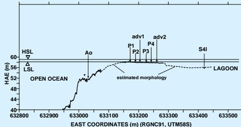
Fig. 2. Reef profile and instrument deployment. P1-4: pressure sensors; adv1-2: ADV velocimeters; S4: electromagnetic current meter; A0: wave and tide recorder.
