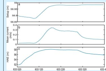
Fig. 5. Computed mean quantities, day 2.3. a : wave setup; b : cross-reef current; c : reef profile
