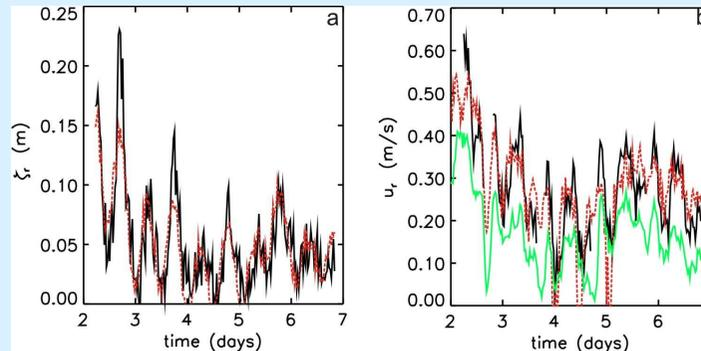
Fig. 4. Comparison between observed (solid line) and calculated (red dashed line, eq. 1 and 2) wave setup  $z_r$  (a) and cross reef current  $u_r$  (b), on the reef-top. Green line: cross reef current in the lagoon at site S4.
